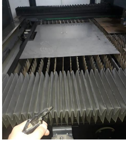
9.5.a Fig. Clening Linear Stage Components
