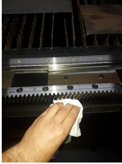
9.5.g Fig. Cleaning Linear Stage Components
