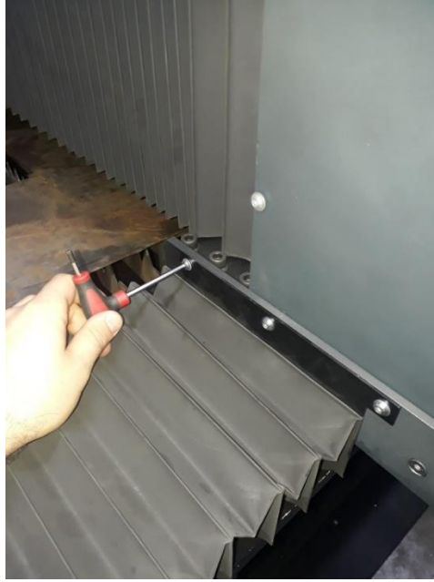
9.5.i Fig. Cleaning Linear Stage Components
