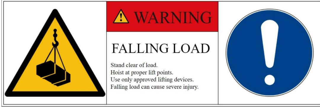
1.1.16 Fig. General Mandatory Action Sign Plate For The Marking Or Lifting Points
