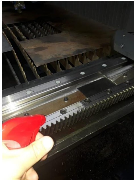
9.5.d Fig. Cleaning Linear Stage Components
