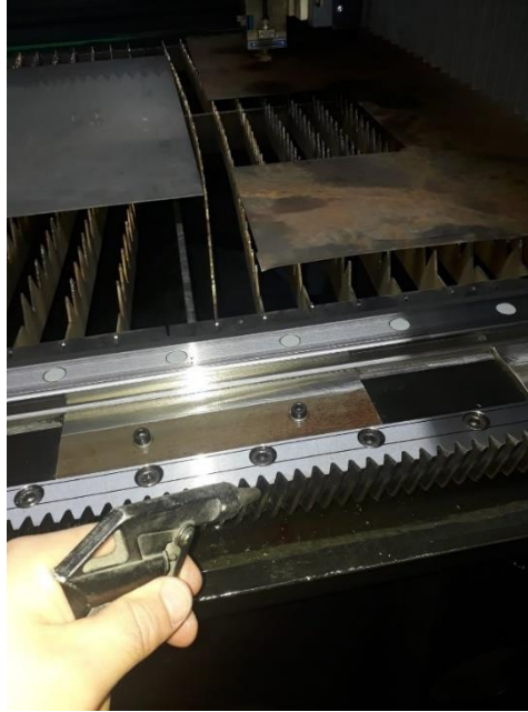
9.5.f Fig. Cleaning Linear Stage Components
