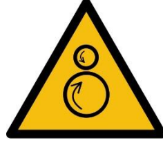
1.1.7 Fig. Counterrotating Rollers
