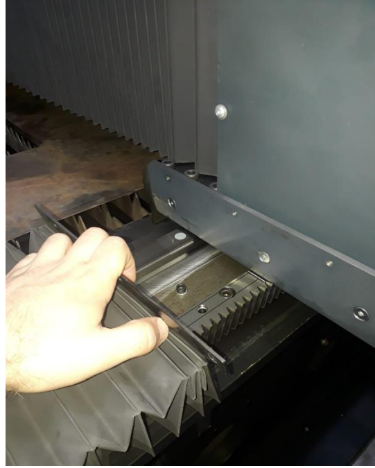
9.5.c Fig. Cleaning Linear Stage Components
