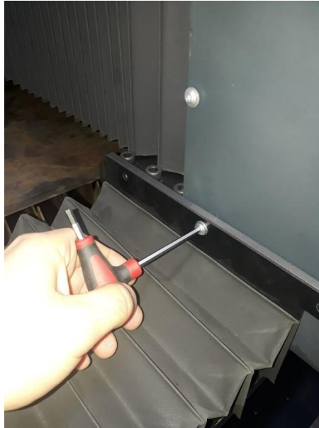
9.5.b Fig. Cleaning Linear Stage Components
